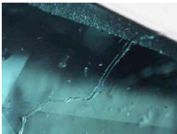
Figure 2a: A faceted emerald held together as one piece by a wide tract of hardened resin as an example of 'emerald with resin'.
