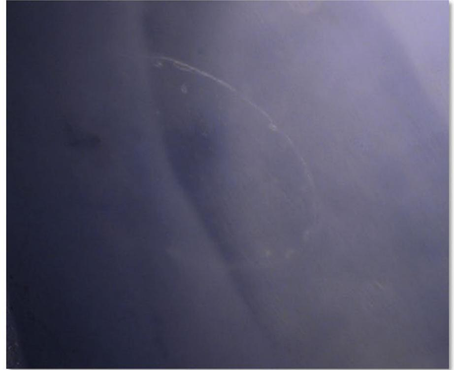
After heating with pressure: Improvement in clarity due to the healing of a narrow-gap fissure.
