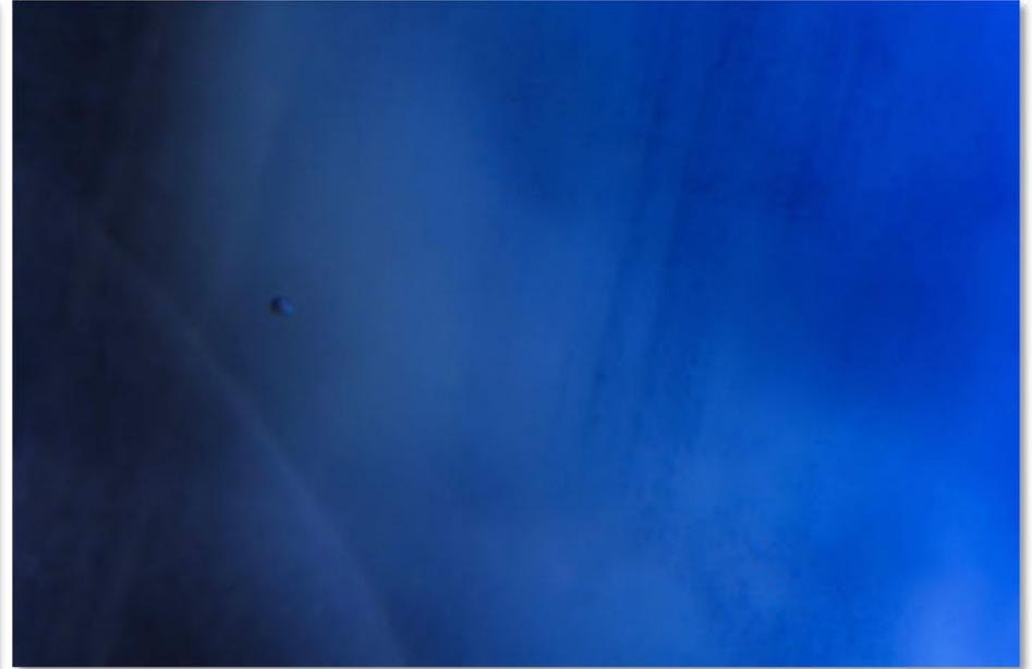
After heating with pressure: Improvement in clarity due to the healing of the narrow-gap fissure at lower left and the halo around the crystal inclusion.
