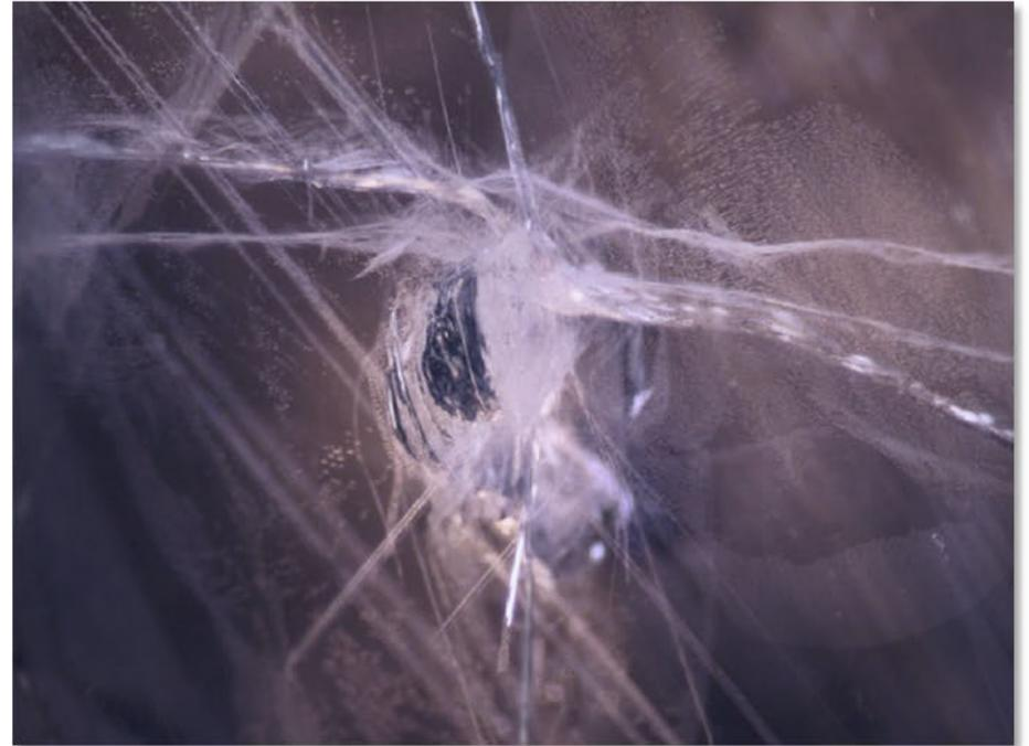
After heating with pressure: Serious deterioration of clarity with new fissures resulting from the treatment.
