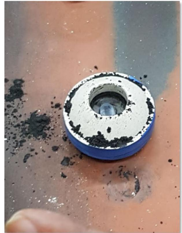
Commonly few drops of water are added into the graphite filled crucible.
